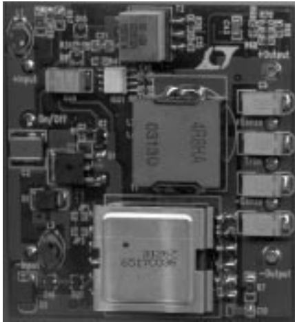
LT1681/LTC1698 36V-72V V_{IN} to 5V/10A Module (See Figure 7 for Application Schematic)
